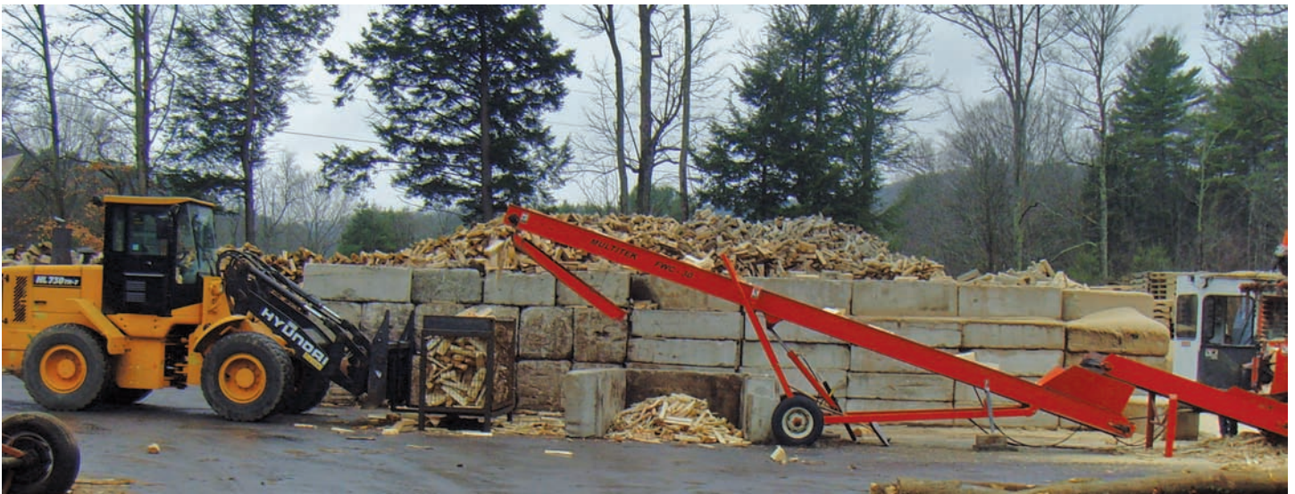
Multitek firewood processor splits the firewood and fills the baskets with firewood to be kiln dried.
