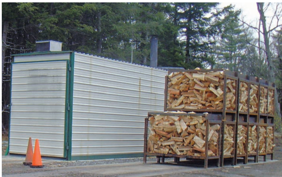
Kiln-Direct MiniQuick firewood kiln with loaded baskets staged for the next kiln charge. Treehugger Farms features value-added kiln dried and debarked firewood.
