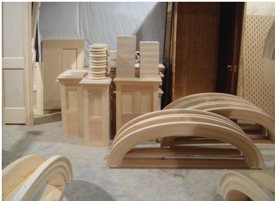
Finished parts include a variety of custom millwork, including moldings and window frames.
