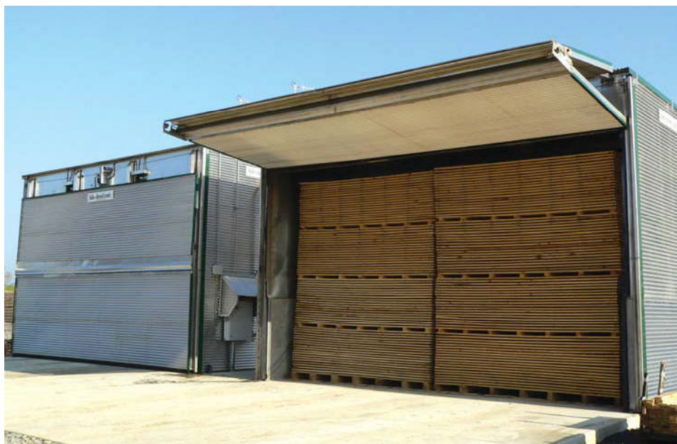
Kiln-direct modular lumber dry kilns, loaded and ready to begin operating, at Cline
