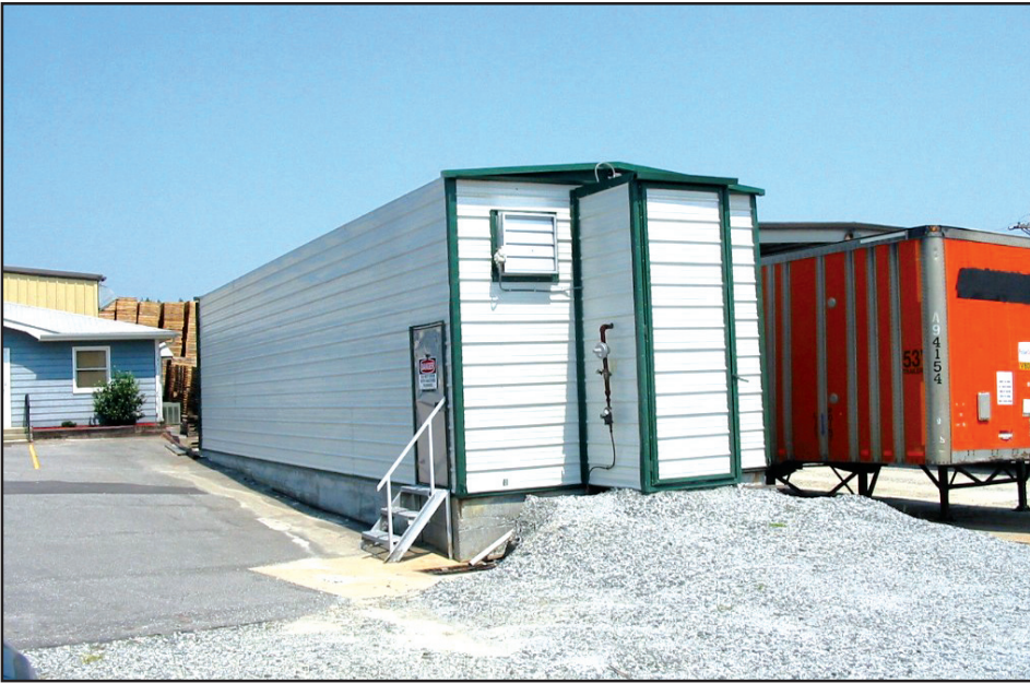
Kiln-Direct heat-treating chamber from rear of chamber.
