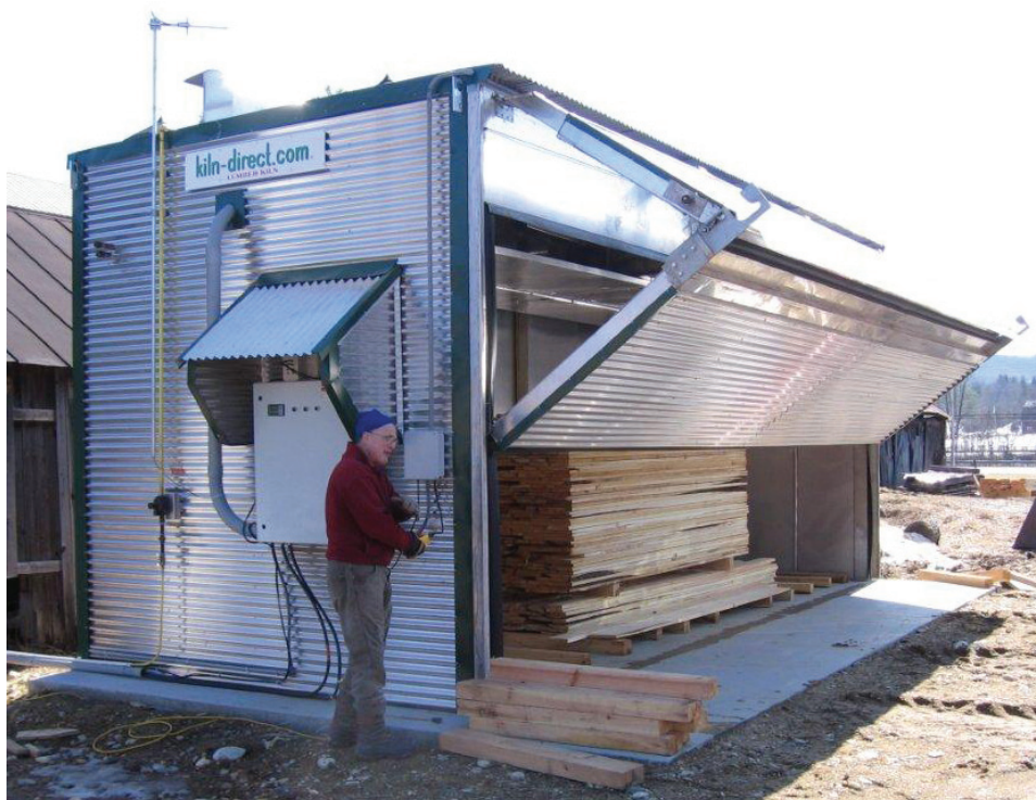
Installation of the Kiln-direct kiln with a front door and sophisticated remote controls has taken drying at The Sawmill at Hall Tavern Farm to a higher level.
