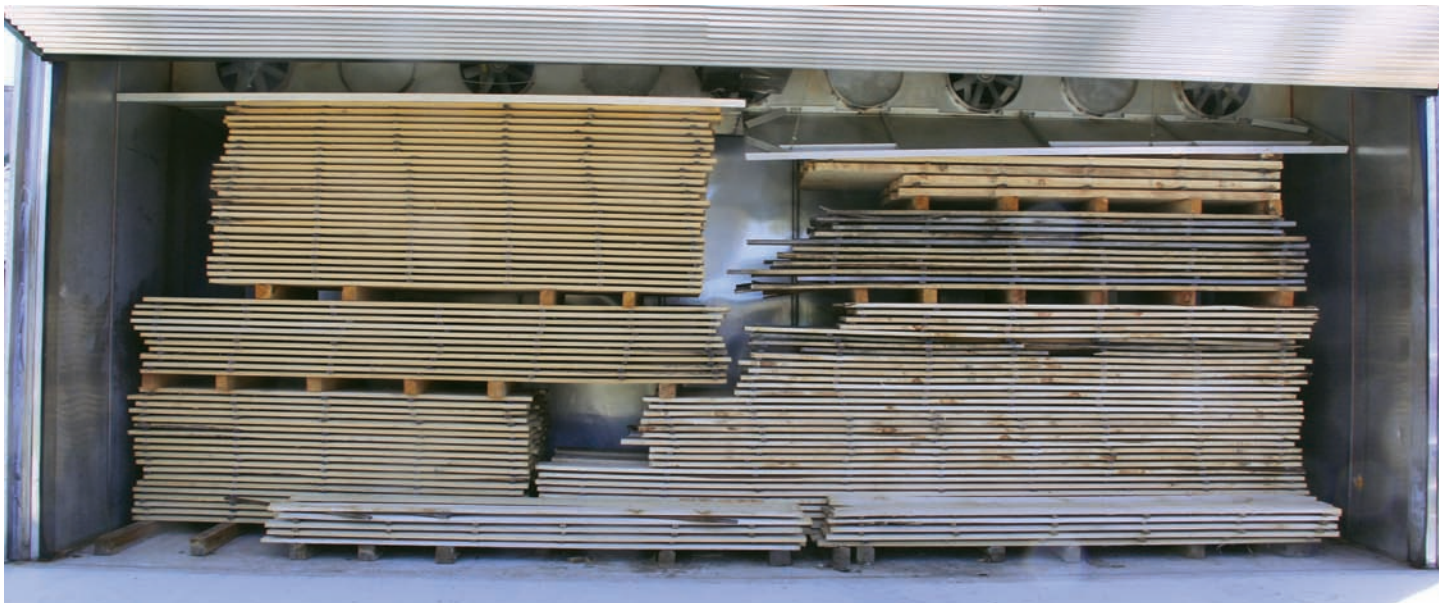
Jay liked the fact that he could get the Kiln-direct lumber drying kiln up and running with propane natural gas fuel and later switch to a wood-waste boiler.
