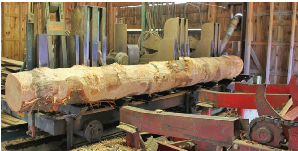
The company uses a semiautomatic mill from Chase, as well as a Chase green chain, turner and edger.
