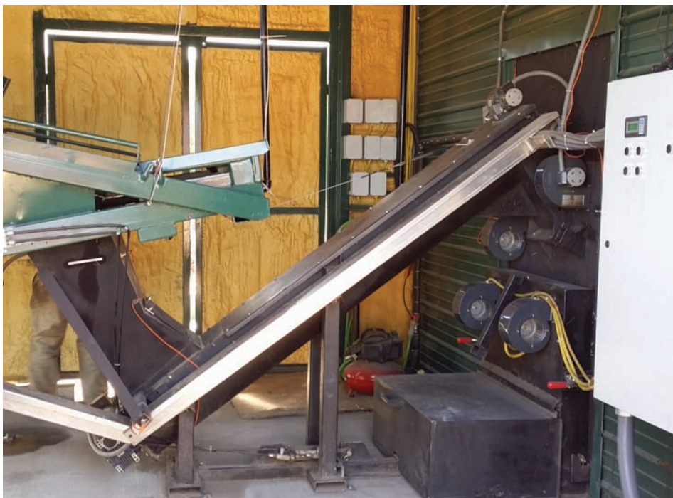
The new SmallQuick kiln uses sawdust, wood waste, or industrial waste, which is stored in the bin (shown above). The bin feeds a funnel that drops wood waste into a screw conveyor that then lifts it up at a 45° angle into the top of the firebox (shown below). Tetreault & Son assisted Kiln-direct by allowing modifications to be made at its site, where this new wood waste system kiln was perfected. This new kiln has been formally introduced to the Kiln-direct product line for 2016.
