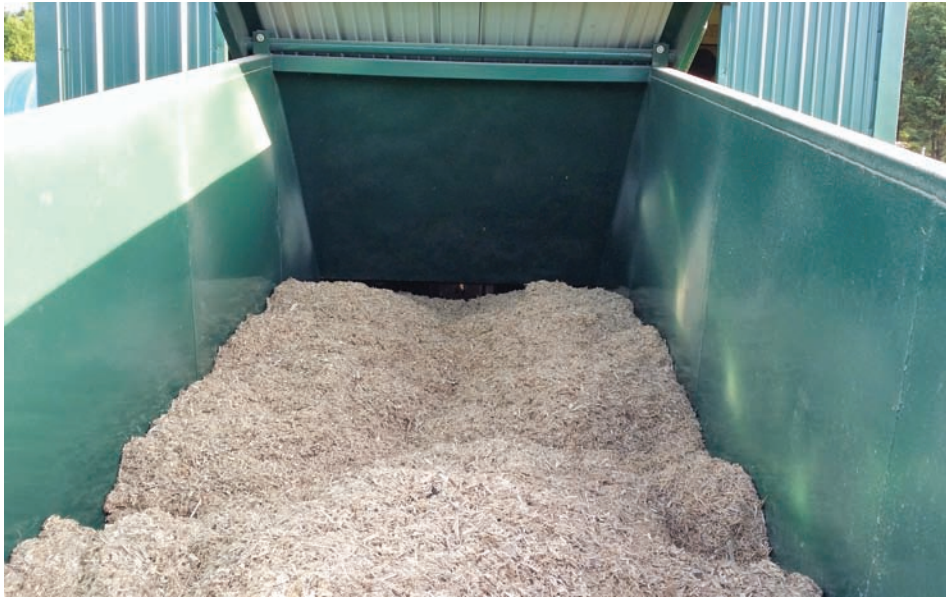
The new SmallQuick kiln uses sawdust, wood waste, or industrial waste, which is stored in the bin (shown above). The bin feeds a funnel that drops wood waste into a screw conveyor that then lifts it up at a 45° angle into the top of the firebox (shown below). Tetreault & Son assisted Kiln-direct by allowing modifications to be made at its site, where this new wood waste system kiln was perfected. This new kiln has been formally introduced to the Kiln-direct product line for 2016.
