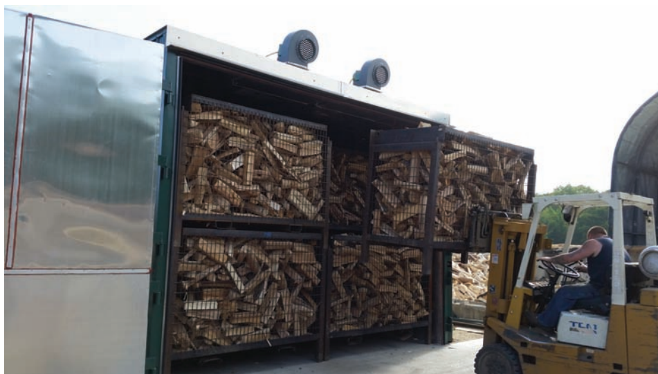
Each of the 24 baskets in the 12-cord SmallQuick kiln hold some 100 cubic feet of loose firewood. Tetreault and Son currently produces 7,500 cords annually of which approximately 6,000 cords are kiln-dried.
