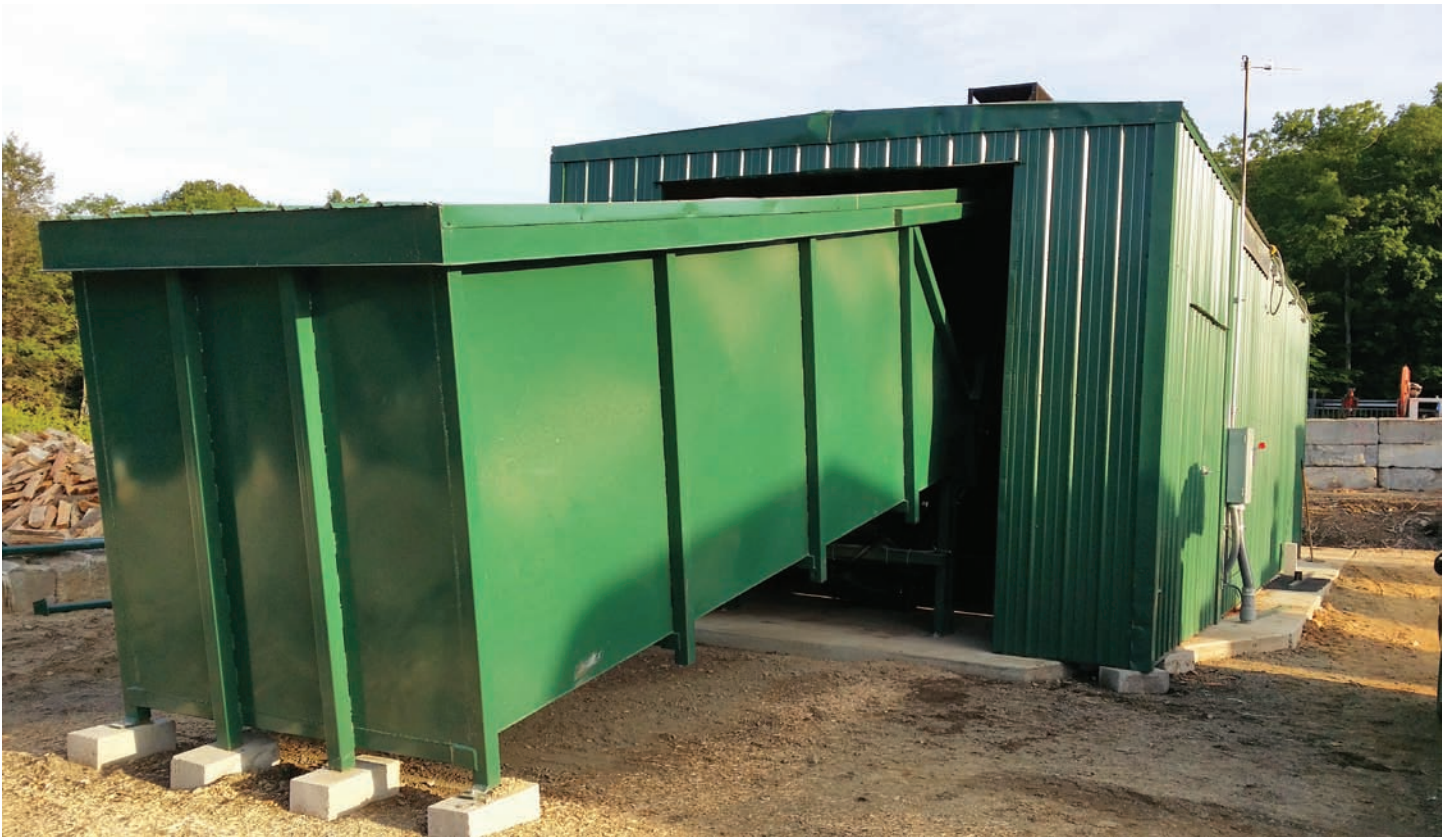
Shown from the back side, the new 12-cord SmallQuick firewood kiln from Kiln-direct features a wood waste storage bin that provides fuel for several days of operation.
