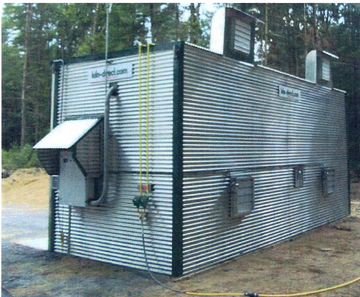
The back side of Drumm's Kiln-Direct kiln illustrates power venting and a heat recovery system that is integrated into the wall, plus a control cabinet on the end. The kiln has computerized controls with an integrated moisture meter that is networked to the office computer for record keeping and kiln management software.
