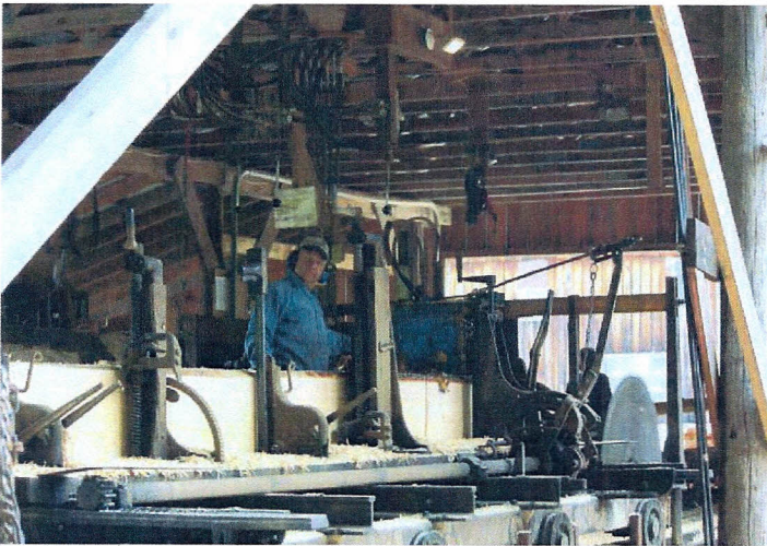
Barney Drumm at the helm of the 50 year old Lane mill, which has a five-knee carriage and is powered by a Cummins diesel engine. The mill runs a 52-inch Simonds carbide-tipped circular blade.
