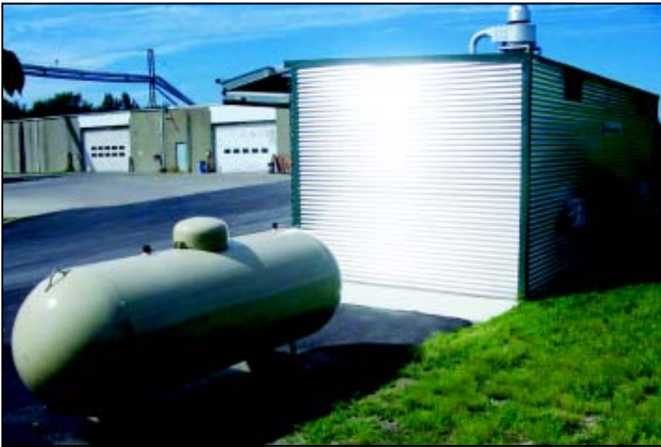
Back side of lumber kiln with LP gas hookup, other heating options available.
